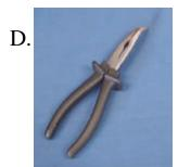
Go inside nozzle with the long nose pliers and, push it into the water tank.
